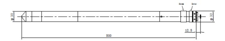
V-ZPL-HITEMP-A-500 is a new High Temp pinhole lens product development. Front optical element is recessed 15mm from pinhole front protects the element for robust longer lens life operating in hot hostile environments.
