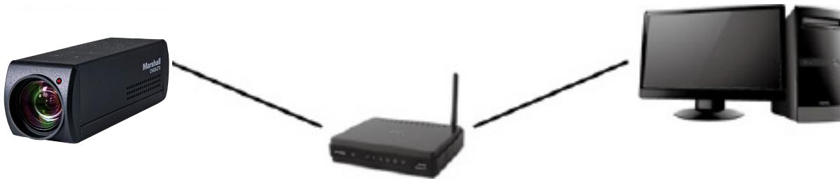
2. If the camera is connected to the computer directly, the computer IP address must be modified to have the same network segment as the camera. For example, the factory-preset default IP address of CV420-27X is [192.168.100.100](http://192.168.100.100). The computer IP address must be set with the same subnet, such as [192.168.100.101](http://192.168.100.101), so that the computer can be connected correctly with the camera.
